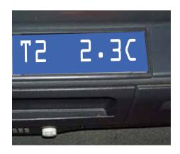
In-cab temperature display unit with driver alert for trailer temperature breaches.
